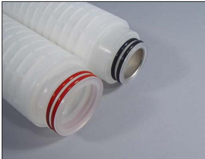
Biopharmaceutical grade Nylon 6,6 membrane filter cartridges are made using Nylon 6,6 membrane. The Nylon membrane used in these cartridges is optimized for retention. Nylon cartridges see broad service in bioburden management for filling operations as well as for buffers, feedstocks, purified water, WFI, and other media. BNM cartridges are also used for the filtration of solvents because of Nylon's broad compatibility and low level of extractables.
