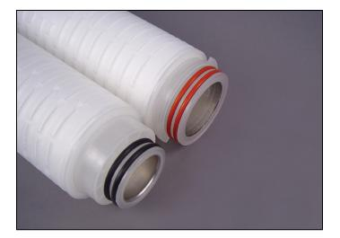
PPD Depth Filter Cartridges are designed to be used as pre-filters in critical pharmaceutical systems. Special attention was given in the design of these cartridges to ensure long life as well as superior retention. PPD Depth Filter Cartridges are rated at 99.9% efficiencies at the rated pore size and have been flushed with high purity water (18+ megohm-cm) to remove any manufacturing debris and ensure particle-free filtrate.
