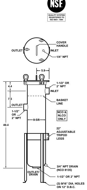
Dimensions are reference only and should not be used for hard plumbing. Consult factory for certified drawings.
