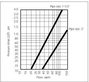
\*Based on housing only. Fluid viscosity, filter bag used, and expected dirt loading should be considered when sizing a filter.
