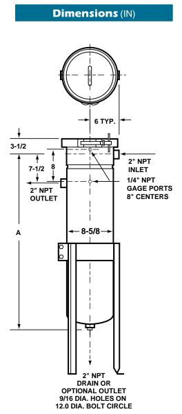
Dimensions are reference only and should not be used for hard plumbing. Consult factory for certified drawings.
