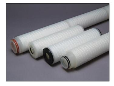
WPS Filter Cartridges with symmetric polyethersulfone (PES) membrane are ideal for purified water filtration. The symmetric membrane used in WPS cartridges guards against bacterial growthrough during the long life of the filter, reducing the potential for biofilm accumulation in system piping. WPS cartridges are flushed with high purity water to remove manufacturing debris.
