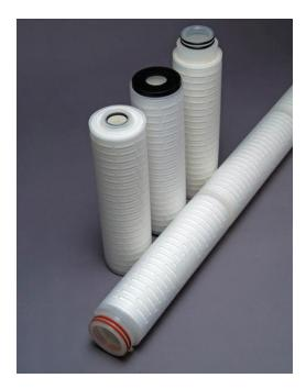
GPVWL filters are made using high capacity hydrophilic polyvinylidene fluoride (PVDF) membrane. High capacity PVDF membrane exhibits high dirt holding capacity, excellent throughput and high efficiency retention. GPVWL cartridges are used for critical prefiltration applications in the processing of a wide range of liquids.
