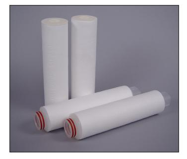
GDMB Melt Blown Media Filter Cartridges are manufactured by a continuous spun-bonding technology that assures a consistent product. The 100% all polypropylene construction gives wide chemical compatibility and extremely low extractables. These cartridges offer exceptional value in both removal efficiency and dirt holding capacity where protection of more expensive membrane filters is important.
