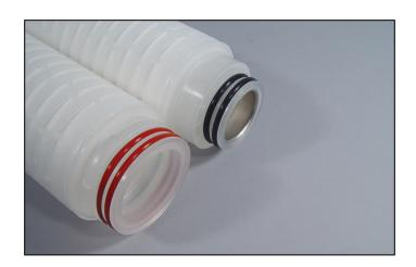
FPVWL cartridges are hydrophilic and manufactured with high capacity PVDF polyvinylidene fluoride (PVDF) membrane. The proprietary membrane casting process creates a thick membrane with high contaminant holding capacity, excellent retention characteristics, high flow rates and low protein binding. PVWL membrane provides excellent throughput and is available in multiple retention ratings to help protect product quality and assure consumer safety.
