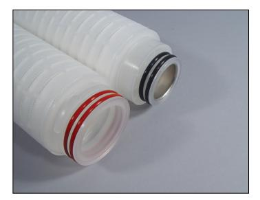
BPVWB Membrane Filter Cartridges are manufactured with high capacity hydrophobic polyvinylidene fluoride (PVDF) membrane. The high capacity membrane provides high dirt holding capacity, excellent throughput and high efficiency particle retention. These cartridges are designed for compressed gas filtration and vent filtration. Representative cartridge modules from each manufacturing lot are tested before lot release from manufacturing.
