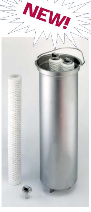
Flow is introduced from above and circulates around  $\triangle$ cartridges. Fluid flows through cartridge walls, leaving contaminant on media, and "clean" fluid exits through bottom outlet.
