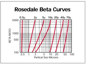
The Beta Ratio (B) at a given particle size can be correlated to the filter efficiency at that particle size according to the following formula:
