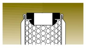
Rosedale seals are not glued onto the cartridge ends as is commonly done. Instead, they are specially shaped to hold in place mechanically, like a grommet. There's little chance they will be dislodged and lost in handling. They are made in different thicknesses to provide seven different standard overall element lengths.
